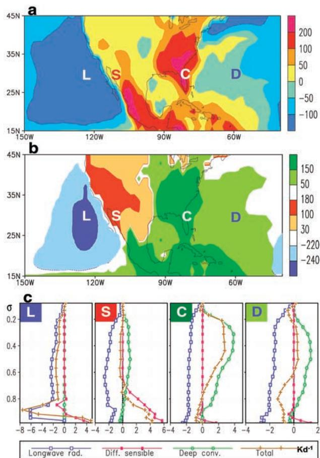
**Figure 1.** July-mean distribution of column-integrated diabatic heating over the PNAA region. (a) Total heating. (b) Main local heating, blue color denotes longwave radiative cooling (LO); yellow and red, sensible heating (SE); and green, condensation heating (CO). (c) Vertical profiles of different heatings at the marked locations L, S, C, and D representing, respectively, those over the LO, SE, CO, and D lobes. Units:  $\text{Wm}^{-2}$  in (a) and (b), but  $\text{Kd}^{-1}$  in (c).
